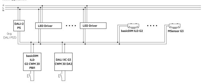
Single / free-standing luminaires, driver with integrated power supply (DALI):
