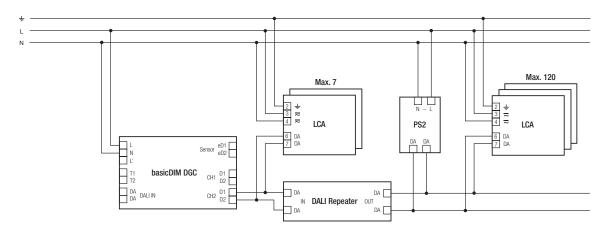
DALI PS1 (24034323), 200 mA, max. 100 additional devices DALI PS2 (28000876), 240 mA, max. 120 additional devices
