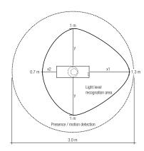
The recommended maximum room height for office applications is 3 m and for corridor applications for example 4 m. Up to 2 m mounting height presence is detected and over 2 m motion is detected.
